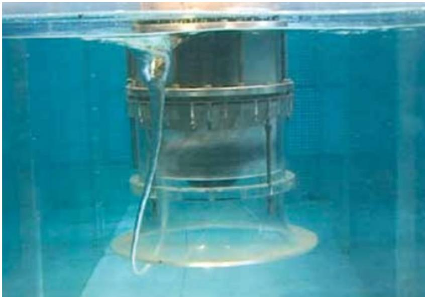
Figura 21 - FSI (Formed Suction Intake)
